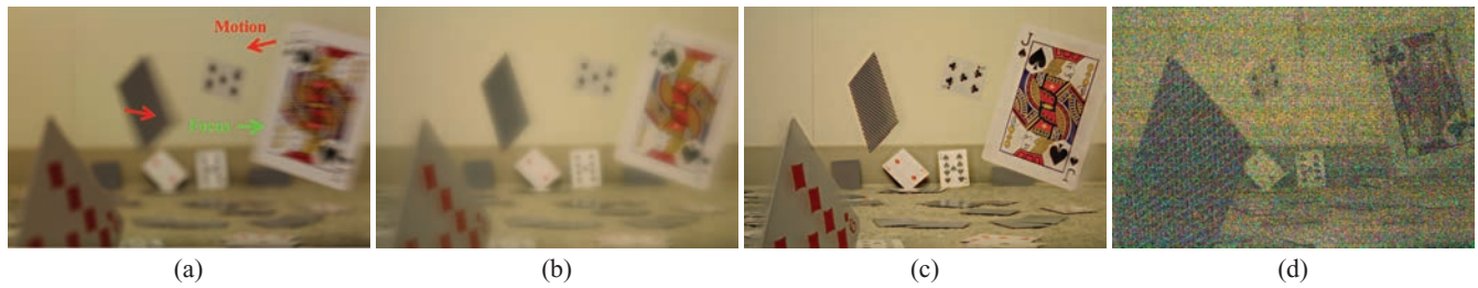
Fig. 13. Playing cards. (a) Standard camera image, focused at the jack on the right; (b) focus sweep camera image; (c) deconvolution result of (b); (d) narrow aperture ( f/36 ) short exposure (5msec) image (contrast-enhanced), taken at a different time instance from (a,b).
